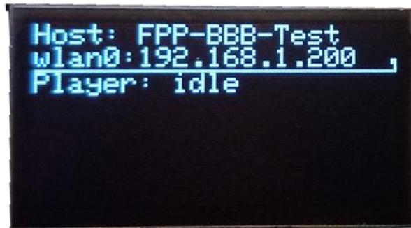
If you press the button on the left, labeled Test/Down, while the OLED display is on the Standby screen then the F8-PB will go into test mode and output a test pattern to the configured output ports. It will display alternating test patterns. It will cycle through a Red-Green-Blue cycle then go to a Red-Green-Blue-White-Off cycle and then turn off and then cycle again. The OLED will show the FPP in testing mode.
