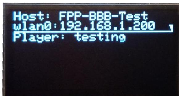
Pressing the button on the right, labeled Enter, while the OLED display is on the Standby screen will open the Status Screen.
