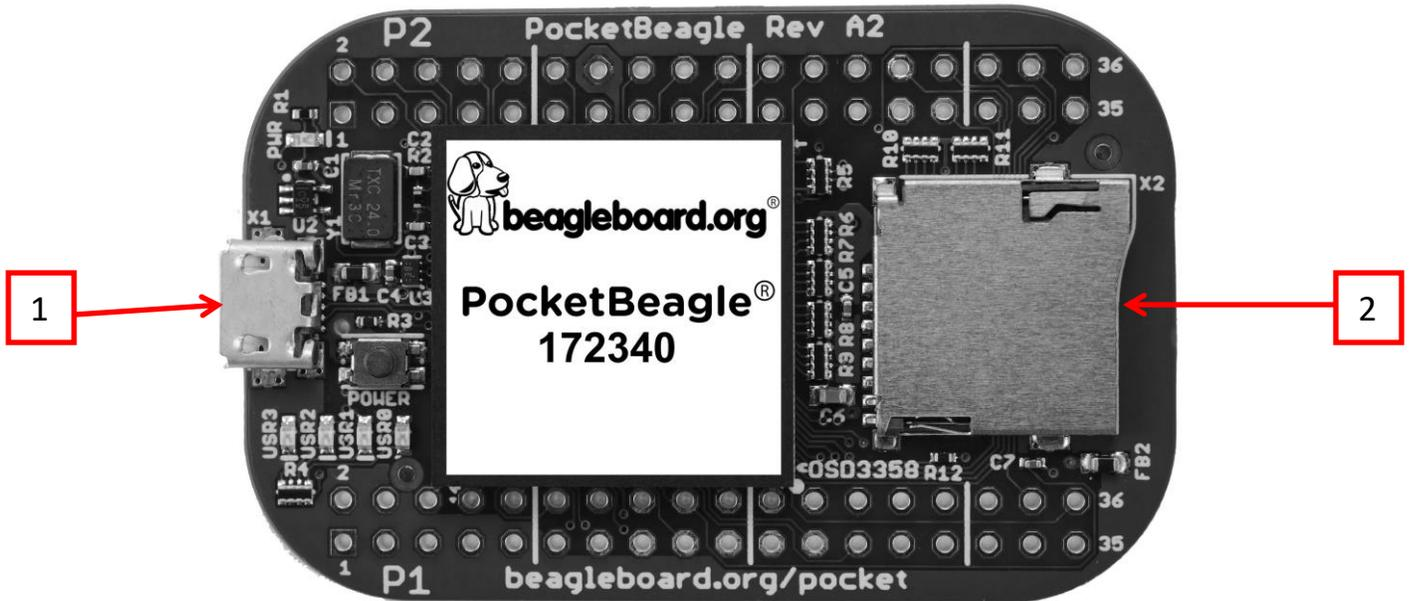
1. Micro USB port- This can be used for the initial installation and configuration of the FPP software.
