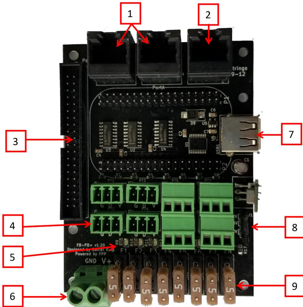
1. RJ45 Multi-Function ports- can be configured for various outputs such as differential expansion, DMX, PixelNet, etc.
