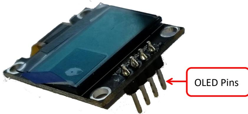
Press the OLED Display onto the F8-PB insuring that all four pins are fully inserted into the header and oriented like the picture below:
