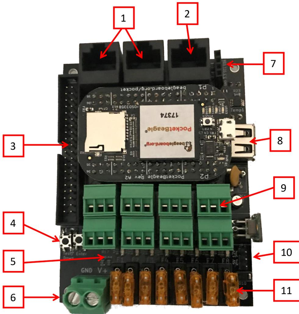
1. RJ45 Multi-Function ports- can be configured for various outputs such as differential expansion, DMX, PixelNet, etc.
